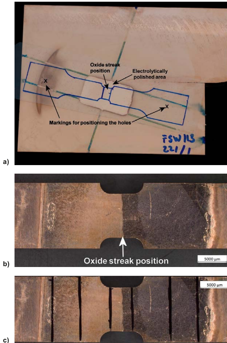
Figure 3-6. Example on positioning the oxide streak in the specimen gauge section. a) A milled specimen FSW113_221_1 that is electrolytically polished in the region of oxide streak. Two markings are made to ensure correct positioning and angle in WEDM-cutting of the specimens. B) A readily cut specimen with an oxide streak perpendicular to the loading direction and c) a specimen with markings for further deformation monitoring.
