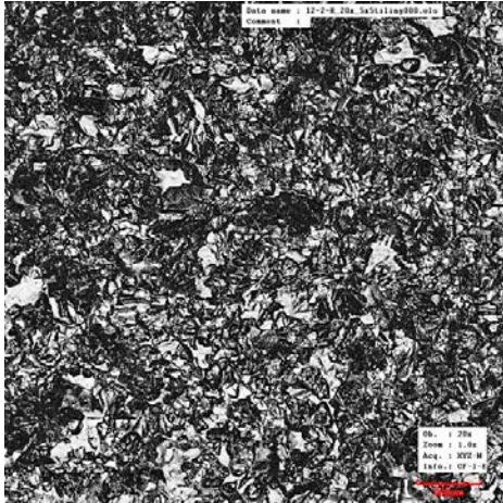
Figure 4-14. Parent material (not weld) from copper sample 112/2. The imaged size is 2.6 \times 2.6 mm.
