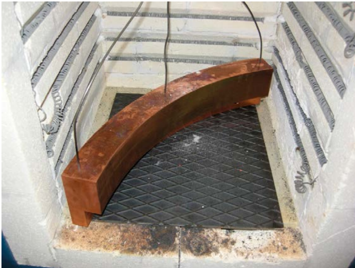
Figure 2-4. Photograph of the dummy sample with inserted thermocouples in the laboratory oven.
