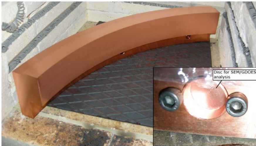
Figure 2-3. Photograph of the segment placed in the laboratory furnace with an insert showing an image of a mounted SEM/GDOES sample.
