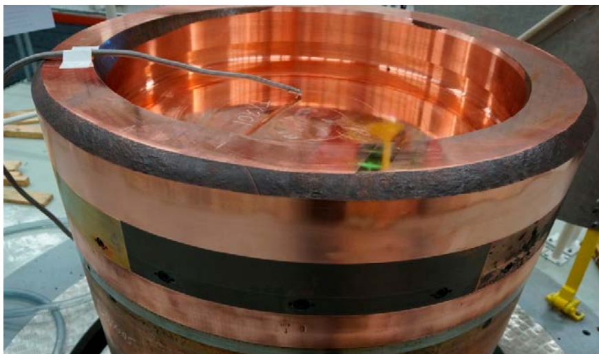
Figure 2-12. A picture of the lid used for welding. Note the radius (black) on the top of the lid. See text for details.
