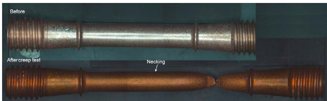
Figure 3-29. Cross-weld specimen from segment 3 (0 \mu\text{m} ) before and after creep testing at 75 ^{\circ}\text{C} and 175 MPa, rupture time 129 h.
