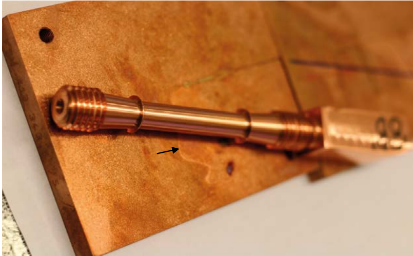
Figure 3-7. Schematic positioning of the cross weld specimens from segment 3 with 0 \mu\text{m} initial oxide layer thickness. The location of the oxide streak is given by the arrow. The metallographic sample is taken from segment 5 with 1.5–1.7 \mu\text{m} initial oxide thickness. The samples were extracted perpendicular to the oxide line.
